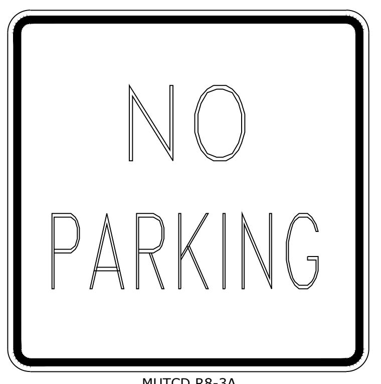
NOTE: SIGNS WILL BE INSTALLED EVERY 100' ON EACH SIDE OF THE ROADWAY CONTAINING A CENTER MEDIAN ON MESA TOP DR.
